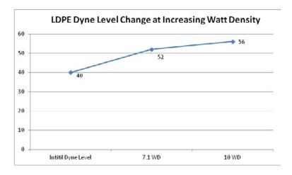
So what are the ramifications of requiring a 7.1 Watt Density? The phycal size and cost of the corona treater increases tremendously. A larger ground roll is required to dissipate the heat created by this higher power level, additional electrode assemblies may be required to achieve the watt density, the air flow requirement for the exhaust system will increase, and of course the power supply will need to have increased capacity as well.
