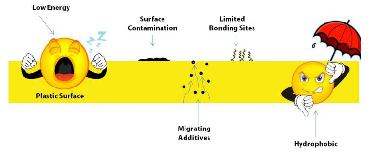
Many corona treater users expect that applying the same amount of treatment to different films will produce the same dyne result. This is simply not true. The first variable is the film's initial dyne level. The second variable is the film's receptiveness to being affected by corona treatment.
