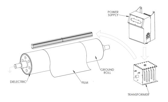
The power supply accepts standard utility electrical power and converts it into single phase, higher frequency (nominally 10 to 30 kHz) power that is supplied to the treater station.
