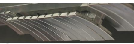
**Segmented** electrodes are used for applications where lane treating or variable treat width is required.
