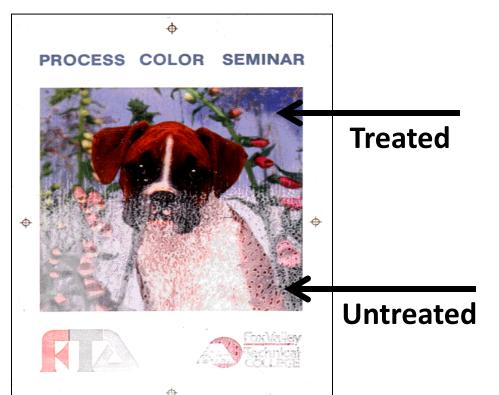
Prior to printing, the upper half of this film was corona treated while the bottom half was not.
