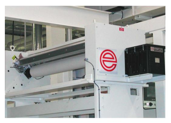
Corona is ionized air created in an air gap between an electrode and ground roll.
