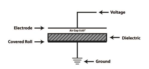
**Corona is ionization of air**. In its simplest form you can think of a corona treater as a large capacitor.
