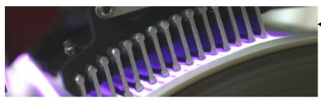
**Fin** style electrodes for fixed width applications requiring higher power treatment and/or ultra wide film width.
