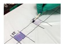
The solution is spread lightly over approximately one square inch of the test material. If the wetting solution stays intact for two seconds, the treat level is at least as high as the dyne level of that solution.
