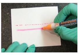
solutions of various concentrations are placed on the substrate until a solution is found that wets out properly. Use an eye dropper style cap to place drops of the test solution from a calibrated dyne-level solution container to the tip of the sterile applicator swab. Use enough solution to coat the tip of the applicator, but not so much that it drips onto the sample. (DO NOT dip the sterile applicator swab as this will contaminate an entire bottle of dyne fluid!)
