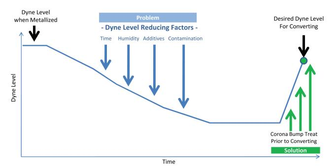
the corona treater not being turned on, to an inability to generate any corona, to a system fault or an application or process issue. It's recommended to always document all of your setup information for each job you run, including power level, line speed and the expected pre- and post-treatment dyne level results.
