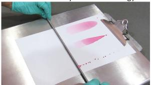
droplets and pulled down. When a film of liquid breaks within the two second period, the tester knows that the treat level of the film is below that dyne solution level. <u>(Watch video of Mayer Rod</u> <u>Drawdown Method.)</u>
