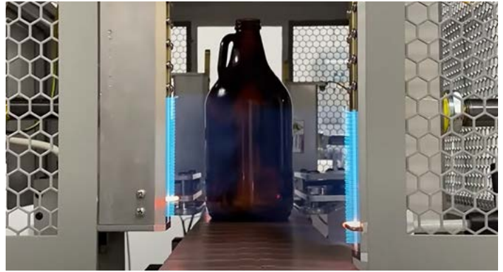
Photo 2. Bottles are treated with two flame-treating heads prior to decorating.
