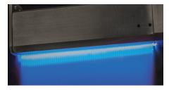
**Flame plasma** is formed when a flammable gas and atmospheric air are combined and combusted to form an intense blue flame. The surface of materials are made polar as species in the flame plasma affect the electron distribution and density on the surface. This polarization is made through oxidation. In addition, functional groups are deposited on the surface.
