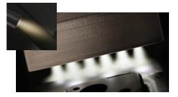
**Blown-arc™** air plasma technology is formed by blowing atmospheric air past two high-voltage powered electrodes and is sometimes referred to as corona treatment. The electrical discharge positively charges the ion particles surrounding it. Through direct contact, these particles positively charge the treated area of the object's surface. This makes the surface more receptive to any applied substance such as inks.
