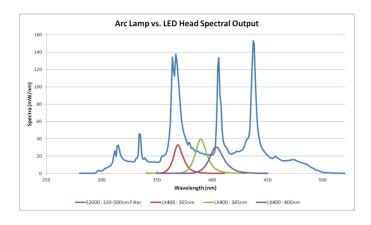
In this case, a 320 - 500 nm filter has been applied to the spectral output of the. The full-spectrum of a mercury lamp will extend from 200 nm and below where it generates ozone, which could be an issue for some applications. It extends into the infrared above 700-800 nm where you can start generating heat from that spectrum.
