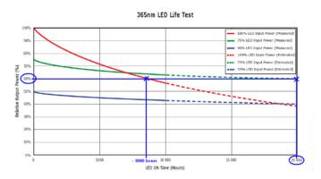
Lamp-based systems typically last three to four thousand hours. The 20,000 hours of an LED is definitely a significant advantage and can help in reducing the running costs for your process. This is another benefit a LED curing process.
