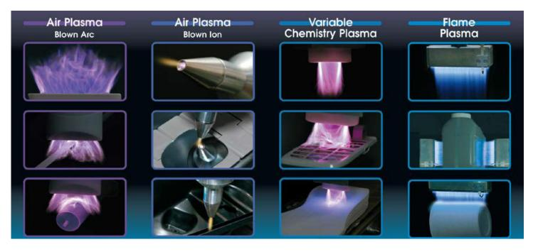
There are a variety of plasma discharge designs which can be employed to meet the geometric and treatment requirements of a specific application. The simplest form of plasma treatment is referred to as a Blown Arc Plasma. It is generated by passing a high-voltage electrical discharge between two electrodes. A single blown arc head treats anywhere from two to three and a half inches and multiple heads can be combined for wider treatment patterns.
