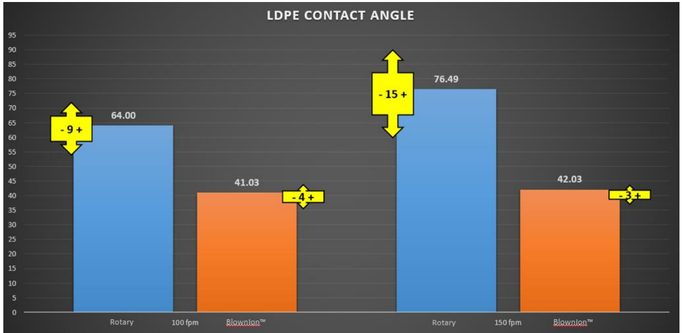
Figure 10 Post Treatment Contact Angle Average and Variation on Low Density Polyethylene (LDPE)
