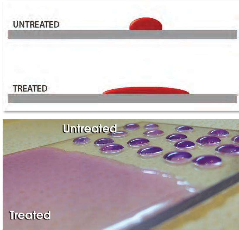
Instant examples of improved adhesion from surface treating can be observed by watching an ink or adhesive droplet wet out on a surface as shown in the examples to the left.
