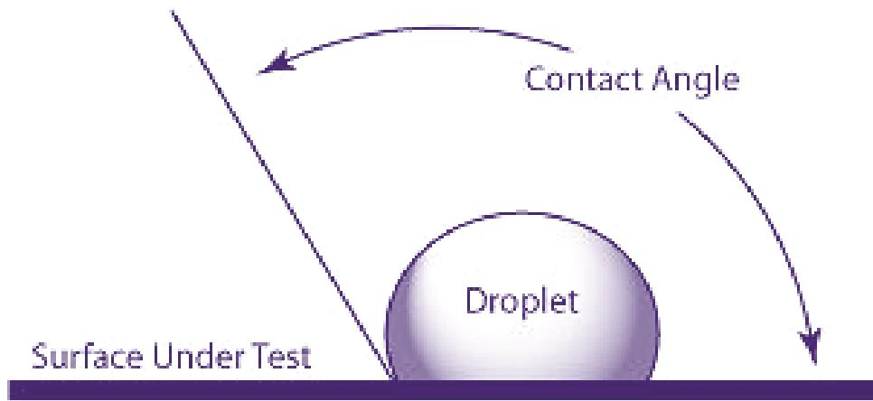
Contact angle measures the interaction of a liquid with a solid.
