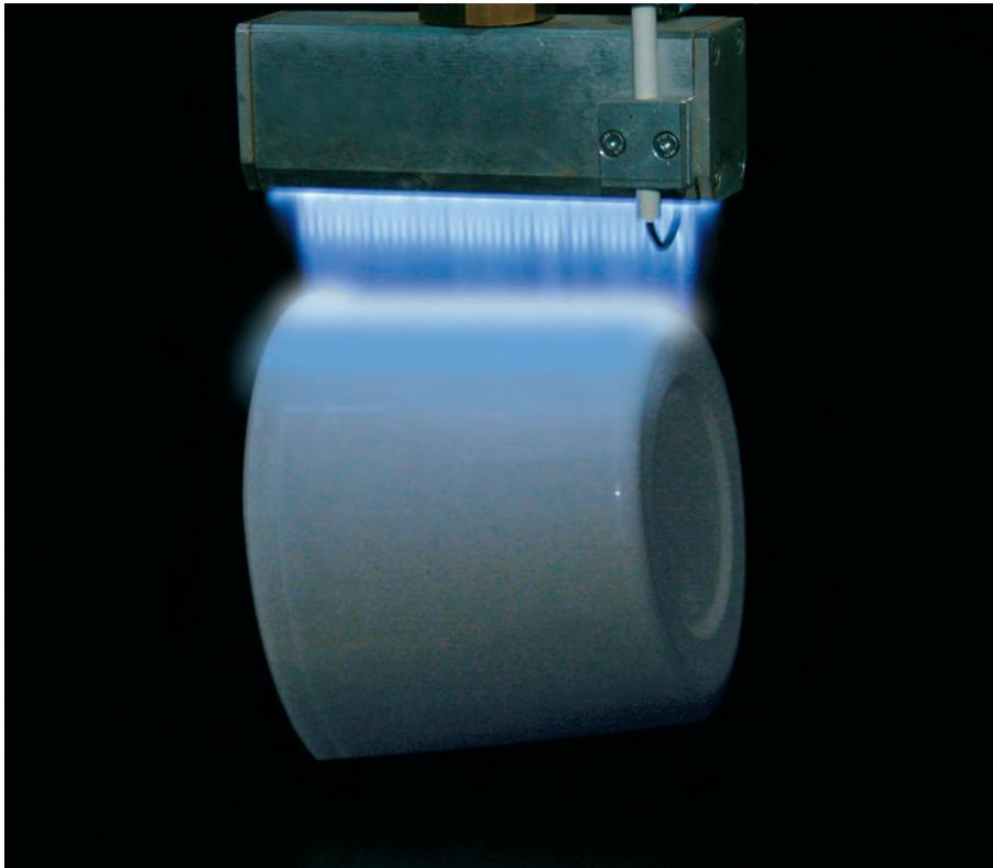
Flame plasma is created when flammable gas and air are combined to combust, forming an intense blue flame.
