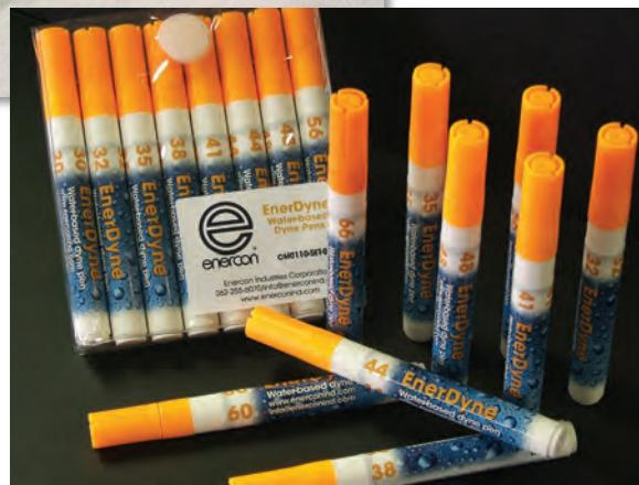
A popular way of determining the effect of surface treatment is to **measure its change in surface energy with dyne solutions.**
