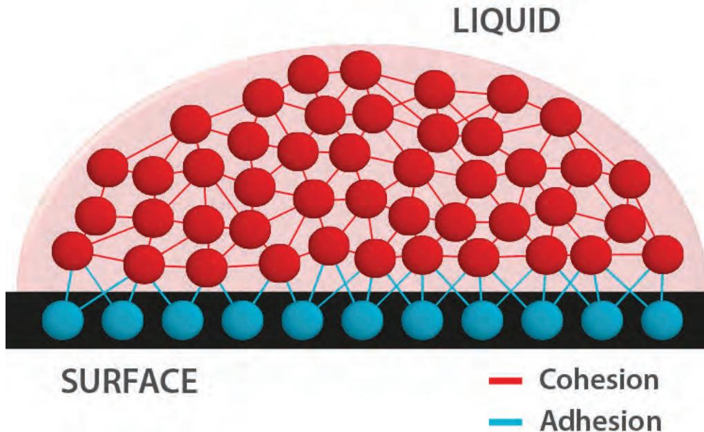
**Low energy, lack of bonding sites, and surface contamination** have a negative impact on molecular attraction, causing liquids to fail to wet the surface.
