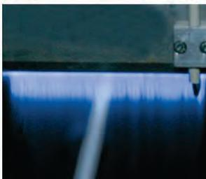
Plasma treatment is being used for a variety of medical applications to clean, etch and functionalize surfaces to improve wettability & adhesion.
