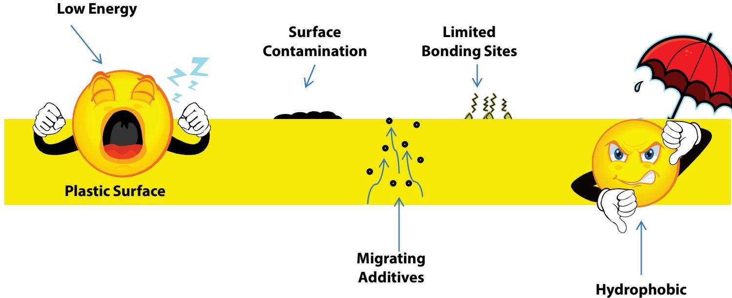
Plastics are generally composed of non polar long-chain molecules with non porous and hydrophobic surfaces. They have low surface energy with few available bonding sites due to low levels of charged ions on the surface. Additionally any type of surface contamination negatively effects adhesion. This includes material additives & release agents which can migrate to the surface
