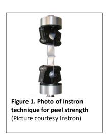
curable adhesive and curing. Peel tests of the TPE substrate coupons bonded to each other with and without flame plasma treatment were subsequently conducted. Peel test results indicated that light curable adhesive 1161-M improves peel strengths when the TPE has been flame treated.
