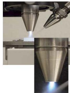
Figure 3. Atmospheric Pressure Plasma Ion Bombardment Device (center) mounted to CO 2 Spray Cleaning Module (right).
