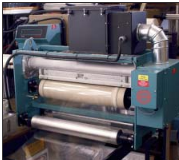
A 24" Universal Roll Treater helps Lofton Label ensure ink adhesion on a variety of films.
