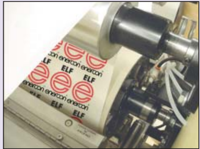
The new ELF (Enercon Low-Friction) Roll adds production stability especially during starts and stops.
