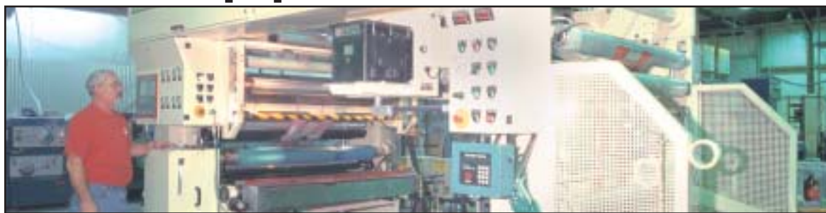
Enercon's corona treating system adds to the productivity of Kendall's 1,000 fpm Schiavi laminator.
