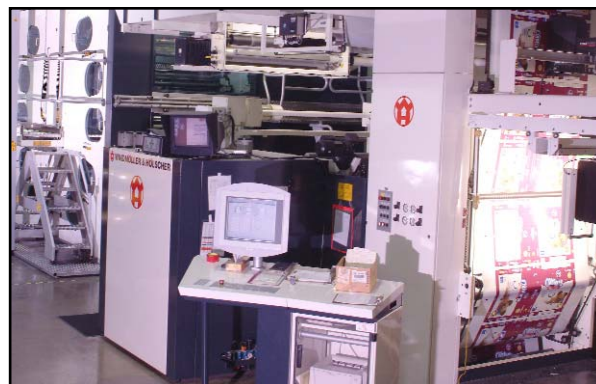
An Enercon treater (top of photo) prepares surfaces for high speed printing on Global Packaging's Novaflex press from W&H.
