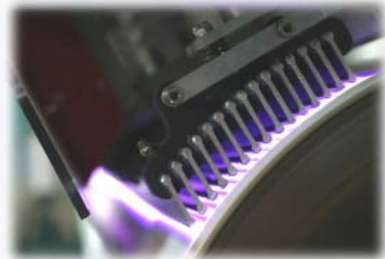
Treatment is a function of power (kW) line speed and web width.
