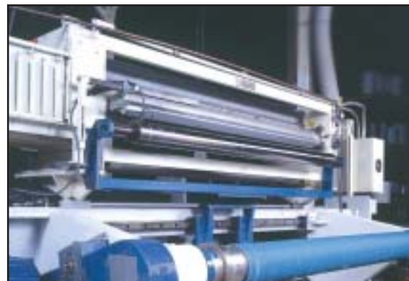
The company relies on an Enercon Universal corona treater for surface treatment.
