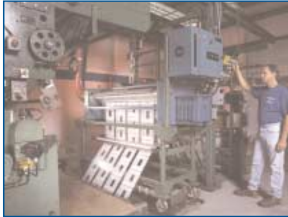
A portable corona treater can be moved between two or more lines for optimal flexibility.
