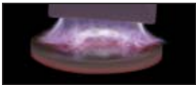
Lids and caps receive treatment to promote adhesion prior to printing and labeling.
