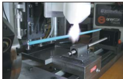
The Dyne-A-Mite™ HP air plasma system prepares medical devices for printing.
