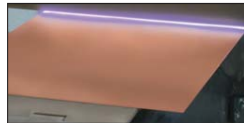
Plasma3™ VCP treats wires (above) and flat object such as sheets and boards (below).
