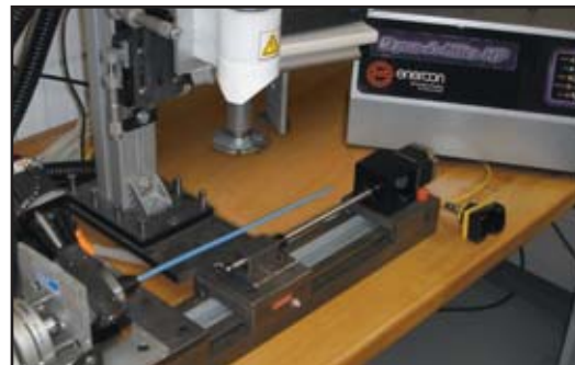
Medical devices precisely rotate and traverse under the treatment head for optimal results.
