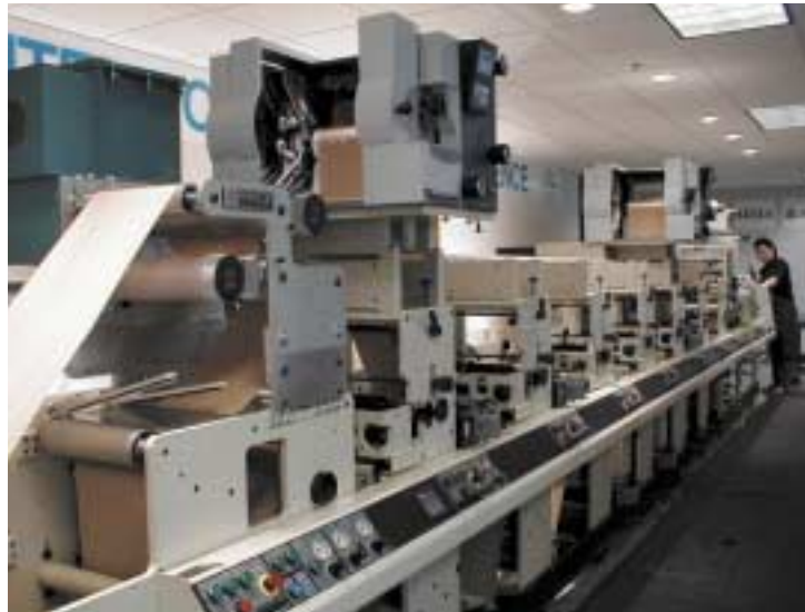
The 4150 Mark Andy press located in Akzo Nobel Inks' Center for Technical Excellence is equipped with an Enercon TL Max II Two-Sided Treater.
