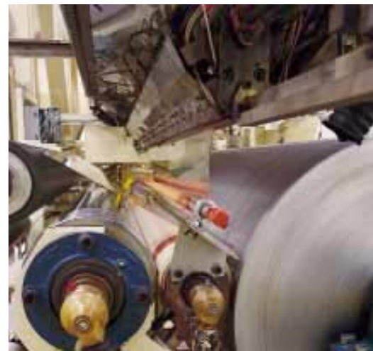
Enercon's Ozonator™ introduces ozone into the nip, enhancing extrudate bonding and increasing production output.
