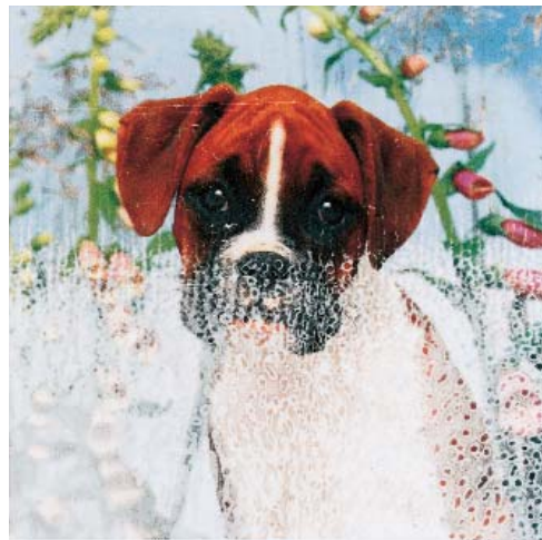
This image shows the flexographic printing results on a substrate where the upper portion was treated and the lower portion was not. The surface energy on the untreated area was too low for the ink to properly wet-out.
