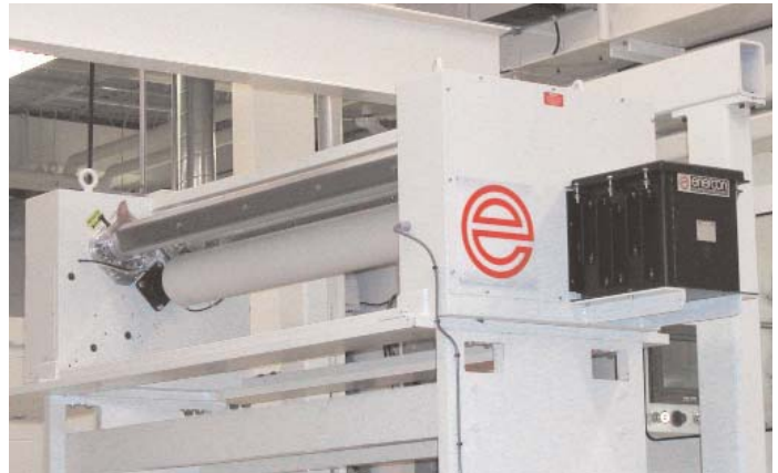
This corona treatment system is designed to produce a larger operating window for flexographic printing operations.
